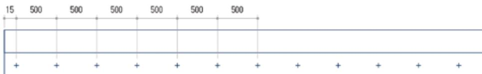
**APPLICATION : PROFIL DE FIXATION POUR COUVERTURE OU BARDAGE. FIXATION HORIZONTALE OU VERTICALE PAR EXEMPLE SUR DES CASSETTES, DES PANNEAUX SANDWICH, DES TÔLES DE BARDAGES,...**
